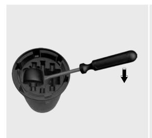
▶ Lever the caster plus its axle out of the slot.
