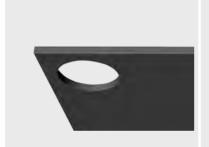
➤ Drill a hole with a diameter of 46.5 mm nto the base plate.
